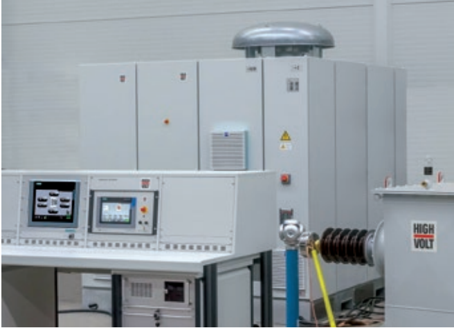
Fig. 1 Test system for type- and routine tests on distribution transformers (left: test voltage source and control system, right: automatic switching system)
